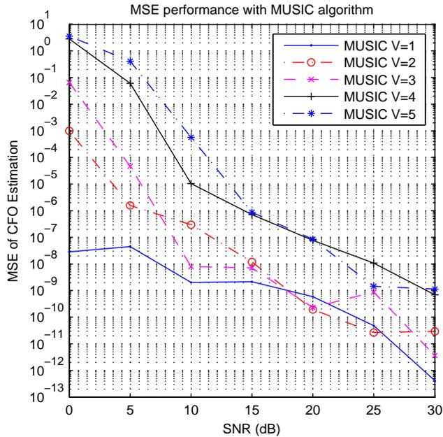
Figure 7: CFO estimation performance of MUSIC (MSE averaged over 2 relay nodes, 100 channel realizations and 250 noise realizations).
