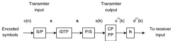
Figure 3: OFDM system block diagram.
