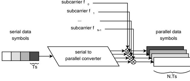
Figure 1: OFDM subcarrier modulation.
