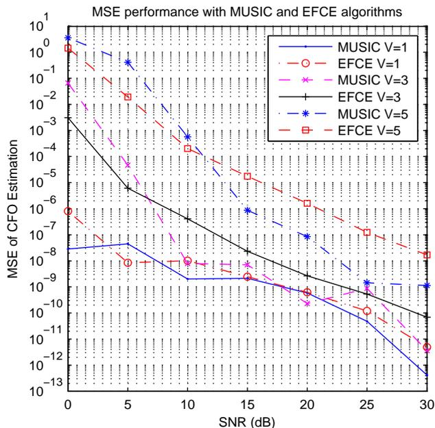
Figure 8: CFO estimation performance comparison between EFCE and MUSIC,  $V = 1, 3, 5$  (MSE averaged over 2 relay nodes, 100 channel realizations and 250 noise realizations).
