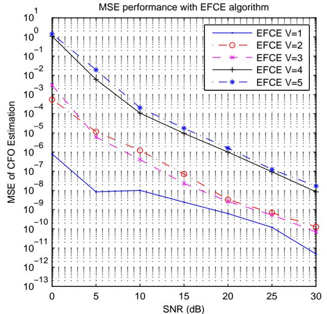
Figure 6: CFO estimation performance of EFCE (MSE averaged over 2 relay nodes, 100 channel realizations and 250 noise realizations).
